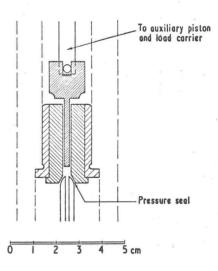
Figure 3. Diagram of piston-cylinder assembly.
